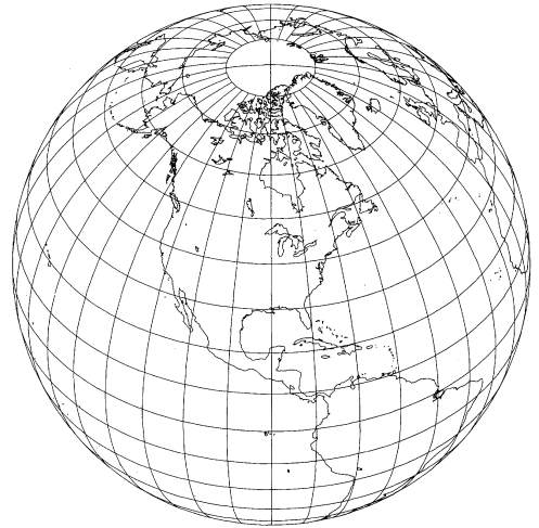
Fig. 1.23 Orthographic projection of the earth showing meridians and parallels at 10^\circ intervals.
